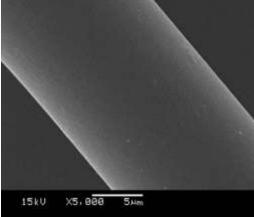
Fig. 2. SEM picture of fibers (5,000X, 15 kV)
