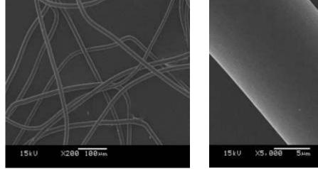
Fig. 1. SEM picture of fibers (200X, 15 kV)
